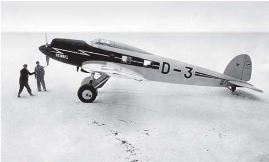
BMW supplied not only the Russian armed forces, but civilian airlines as well. Lufthansa's He 70 high-speed passenger plane was driven by a BMW VI.
