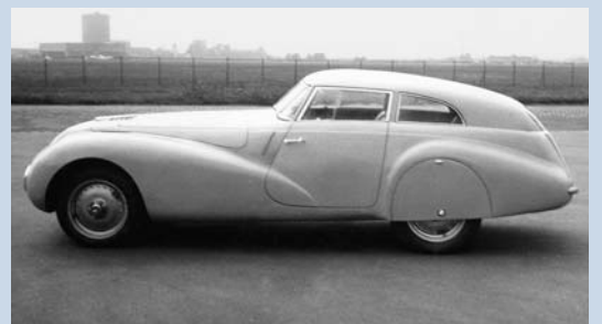
The tubular space frame for the AM 1008 Kamm Coupé (left) was made of electron and weighed just 30 kg. The up-and-running Kamm Coupé (right) during testing at the Oberwiesenfeld airfield.
