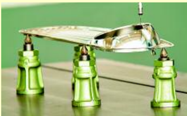
There is a complex and often long-drawn-out process involved in making an "old" spare part available. This picture shows a front trim grille being manufactured for the 02 Series on the basis of old documents. The process uses new engineering techniques to press out the grille, and compliance with the specified dimensions is checked automatically.
