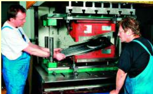
There is a complex and often long-drawn-out process involved in making an "old" spare part available. This picture shows a front trim grille being manufactured for the 02 Series on the basis of old documents. The process uses new engineering techniques to press out the grille, and compliance with the specified dimensions is checked automatically.
